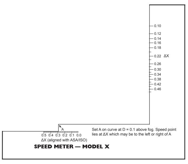
To align with ASA/ISO speeds, the speed obtained by this meter is 0.29 "to the right" of the speed called "delta X speed." Derived from the 1955 paper by C. N. Nelson and J. L. Simonds of Kodak Research Labs, Simple Methods for Approximating the Fractional Gradient Speeds of Photographic Materials.
