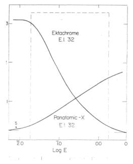
Fig. 10. The density vs. log-exposure curves for Kodak Panatomic-X and Kodak Ektachrome Films used in the present study.
