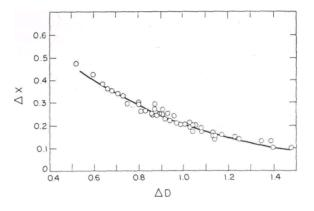
fig. 13. Data for a number of different films and various development conditions showing  $\Delta X$ plotted against \_a.o. where  $\Delta X$  is the log f difference between the exposure at a density c 0.1 above fog and the exposure at the fractional-gradient speed point.
