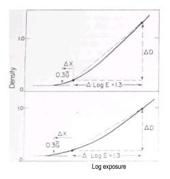
Fig. 12. D-log f curves showing the inverse relation between  $\Delta D$  and  $\Delta X.$   $\Delta X$  increases when  $\Delta D$  decreases.
