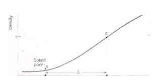
Fig.2. The D-log E curve for a negative film, showing the location of the exposure,  $E_a$ , for the gray object measured by the exposure meter.
