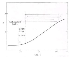
Fig. 7. The log E positions of the negatives exposed as prescribed by a calibrated exposure meter used with the ASA exposure index of the film.
