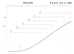
Fig. 4. The D-log E curve for the film used in the experimental study of the safety factor. Dashed lines show the log E positions of the six camera negatives for Scene 1.
